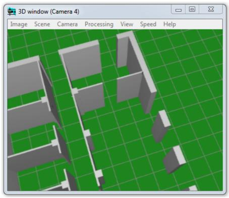
Fig. 5. Walls have been created. The view in 3D window from Camera 4 lifted on 15m. height.
