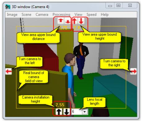
Fig. 16. PTZH frame in the 3D window.
